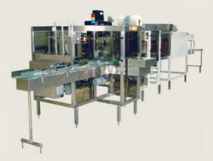
Fully automatic tray erecting and gluing, product collation and loading
